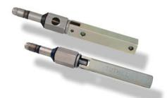
THV, TH, and TK Quick Connectors are designed for testing and filling copper tubing, such as that used in refrigeration coils. They are particularly useful in applications where the length of tube extending out of the header plate is not long enough to permit the use of a standard O.D. retaining tube connector. Construction materials include stainless steel, hardened and plated carbon steel and neoprene seals.
